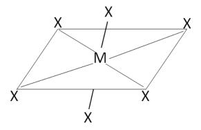
Figure 5. Tetragonal compression or Z-in distortion
