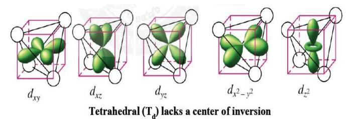
Figure 3. Splitting of d-orbitals in Tetratahedral Field
